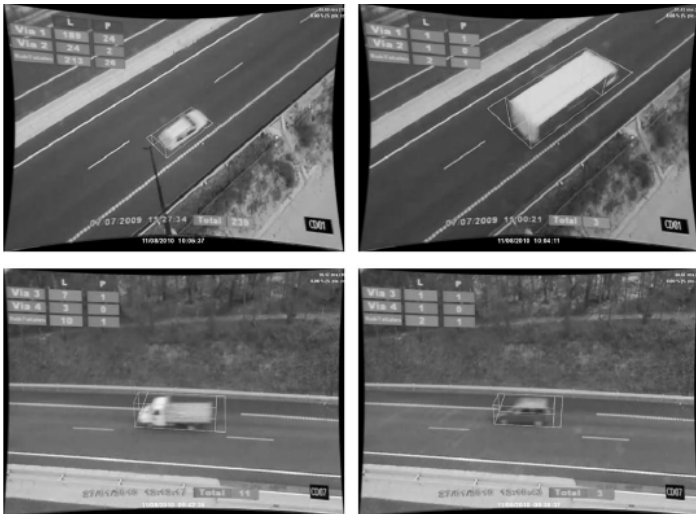
Fig. 2. Some samples of 3-D tracking result [1].
