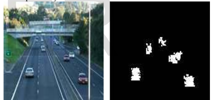
Fig. 4. Background subtraction on a low definition image ( 128 \times 160 ).
